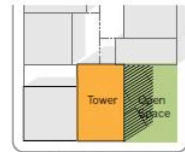
b. DO NOT - Place tower directly south or west of open space
